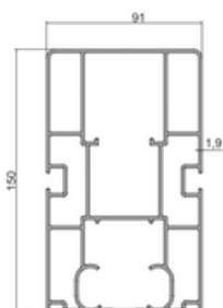
Standard Serie Guide Rail - 5,217kg / m 91mm x 150mm
